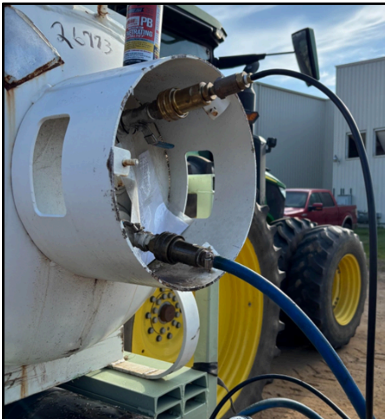
SUPPORT HOSES AND AVOID SIDE-LOAD ON FITTINGS.
