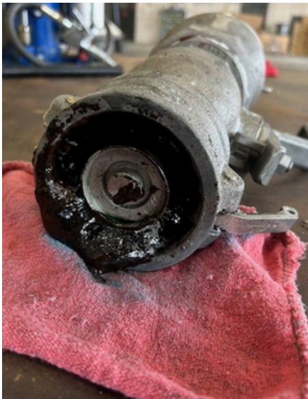
Aluminum valve with TELONE™ residue left inside.
