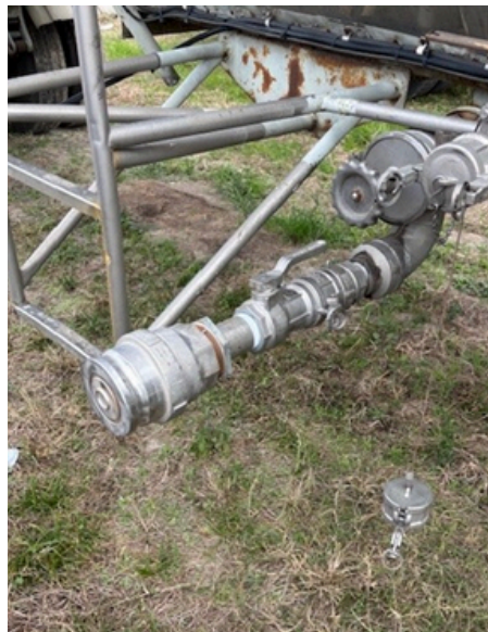
Stainless steel custom adapter for loading.
