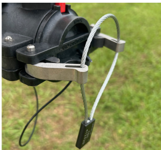
Metal cable seals used on tanker trailer valving when transporting TELONE™
