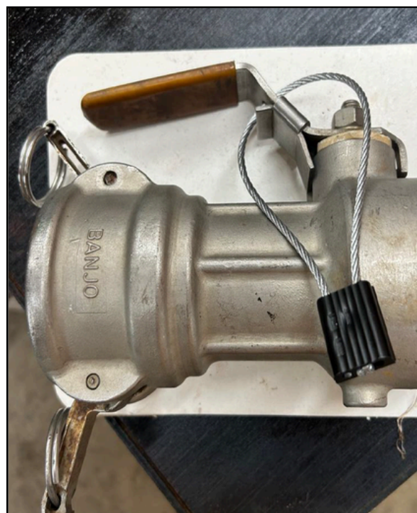
Metal cable seals used on tanker trailer valving when transporting TELONE™
