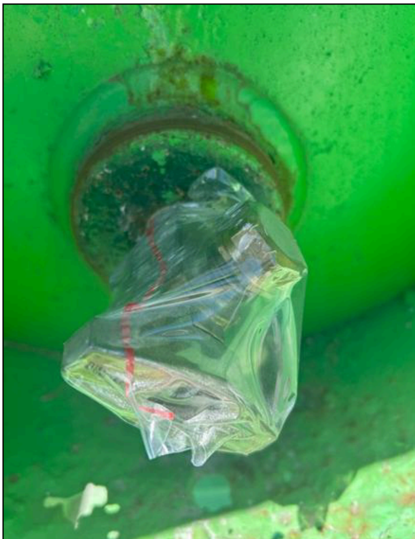
Plastic heat shrink wrap over a cylinder valve used in TELONE™ handling
