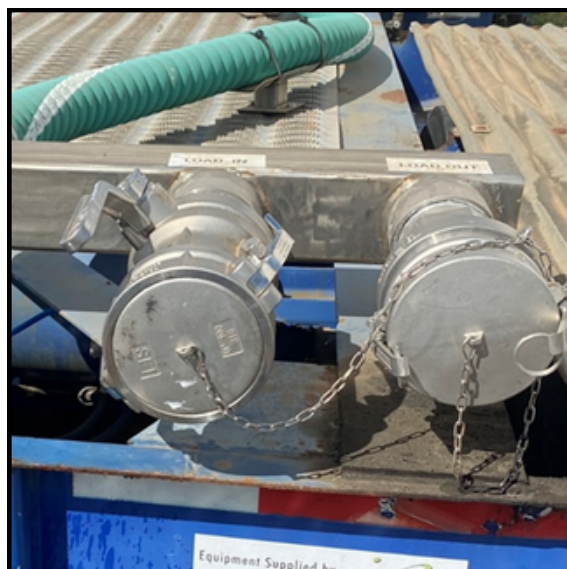
SAFETY CAPS ON VALVES ON A TANKER
